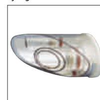
Sylfog -50°C: one silicate glass ø38 mm internal tube, and a ø50 mm internal polycarbonate protective one, electrical equipment and starter for standard 36W and 58W lamps.
